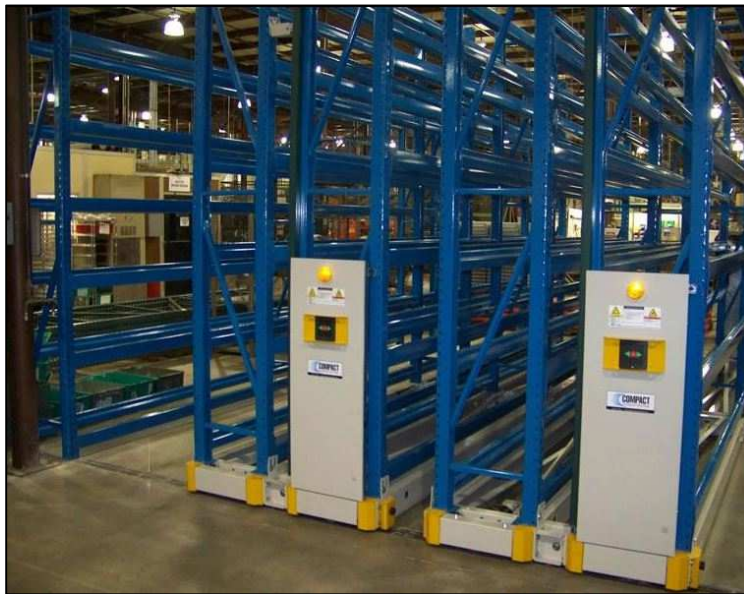
Image 3. Vertical Mobile Racks
